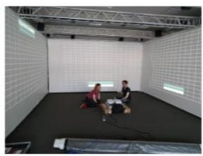
point for experiments. The truss holds stage lights, studio speakers, microphones, tracking sensors, various cameras (depth, high-speed, or thermal), and projectors. This set-up allows very diverse experiments and scenarios like caves, ambient lighting, 360° sound, recognition of emotion, faces, gestures, or speech. Our infrastructure is based on:
